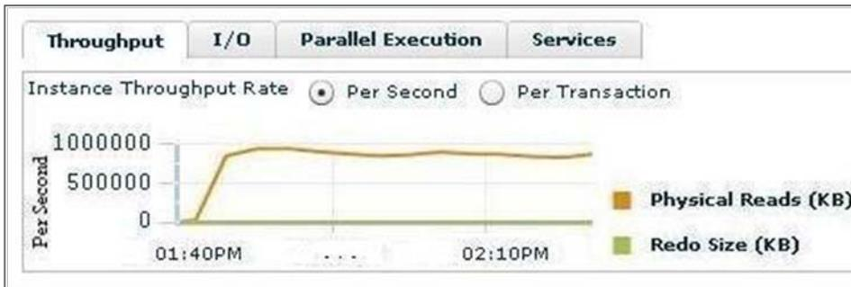
Figure 9 shows the total throughput of our eight-node database approaching 8,000 MB/s and leveling off for the duration of our test measurement interval. The data represented here is consistent with the data presented in Figure 5.
