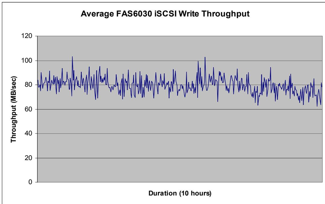
Figure 13) Average FAS6030 iSCSI write throughput.
