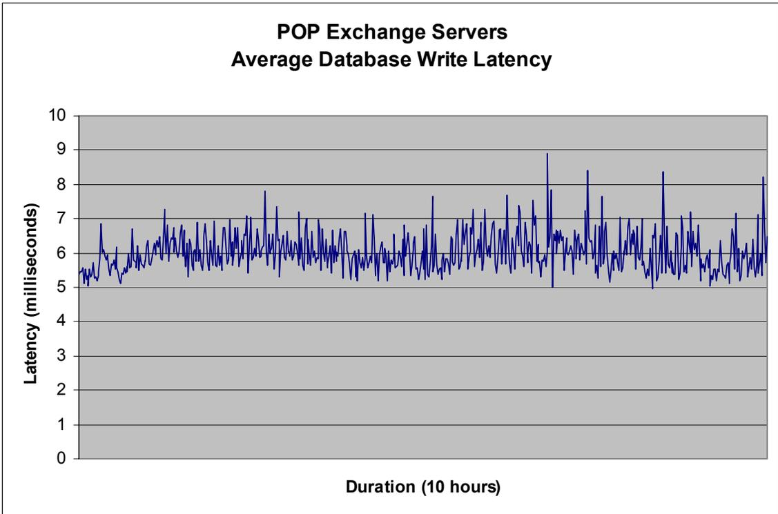
Figure 7) POP Exchange Servers average database write latency.
